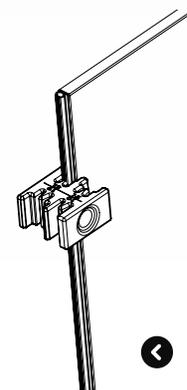
Seal application tool in-situ on a 12mm glass door panel
